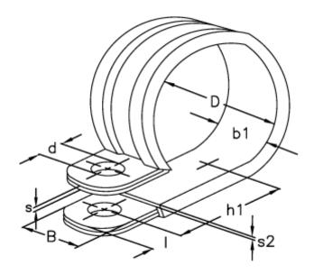
$\begin{array}{lll} b1 & = 31.0 \\ d & = 10.5 \\ Diameter D = 75 \\ h1 & = 55.0 \\ I & = 10.0 \\ s & = 1.25 \\ s2 & = 3.0 \\ Width B & = 25 \\ \end{array}$
